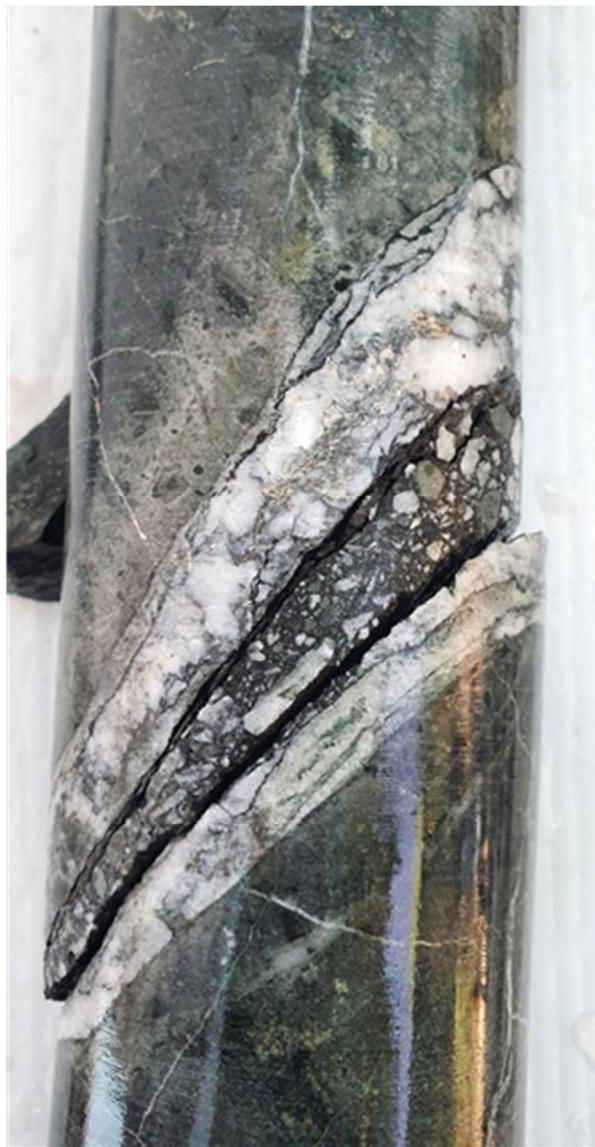
Figure 5. Close up of NQ-sized core (4.8 cm diameter) from Hole BA23-57 with Native Silver vein grading 6,440 g/t Silver over 0.2 metres. Note threads of shiny metallic Native Silver in the upper vein zone and the black acanthite (silver sulphide \text{Ag}_2\text{S} ) filling breccia in the middle of the vein. This is the style of mineralization seen historically in the district approaching major mineralized shoots.
