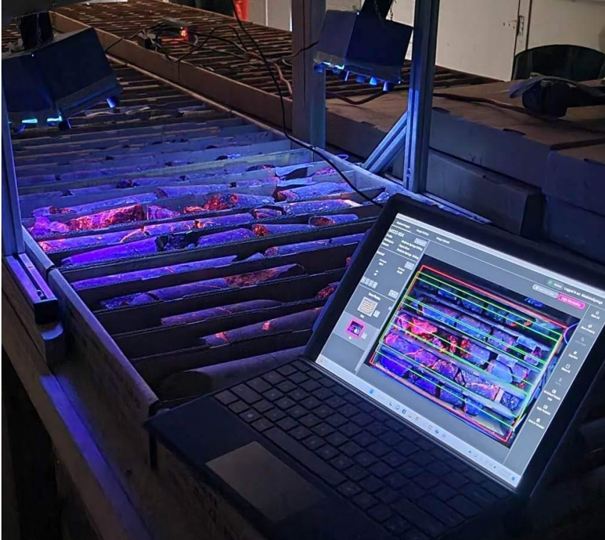
(Left) Fluorescence spectroscopy setup for drill cores; (Right) Fluorescent veins in MS22-001 core
