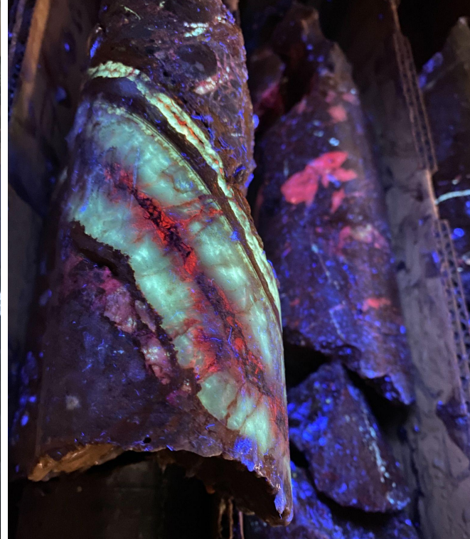
(Left) Fluorescence spectroscopy setup for drill cores; (Right) Fluorescent veins in MS22-001 core
